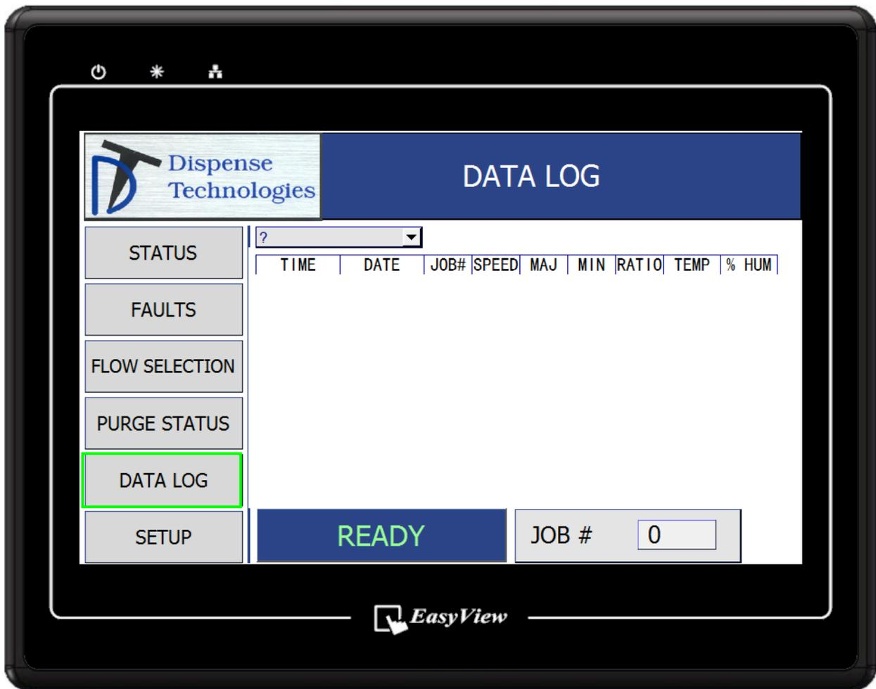
OPTIONAL: The data log screen shows the data logged while the system is running. The **JOB NUMBER** can be entered and used to log data to a specific job number from 0 – 9999
