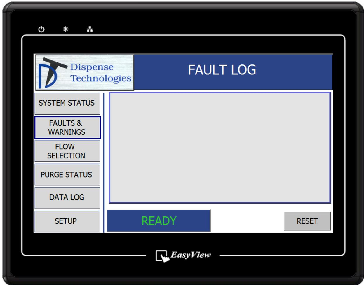
The Faults and Warnings screen will indicate and log any faults or warnings with a time stamp while the machine is on. The log is reset when power is turned off.
