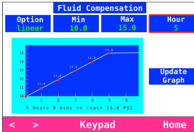
Figure 4-17: Pressure Curve for Sample Linear Program
