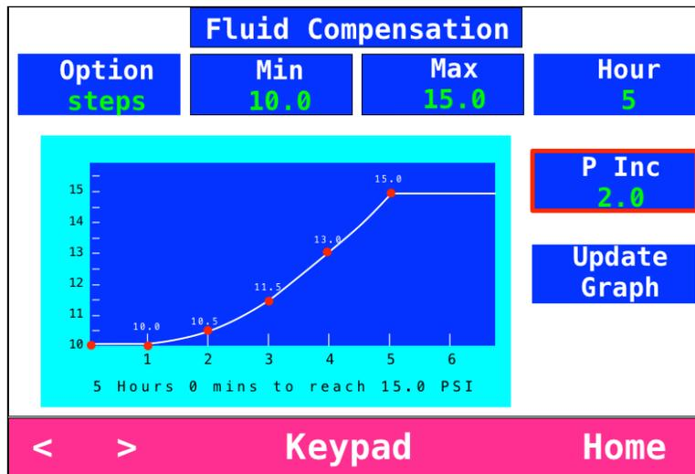
Figure 4-18: Pressure Curve for Sample Steps Program
