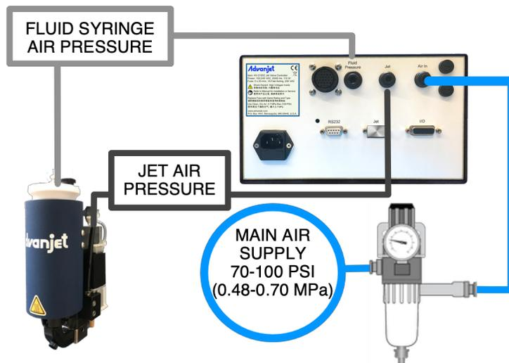
Figure 2-1: HM-2600C Pneumatic Connections
