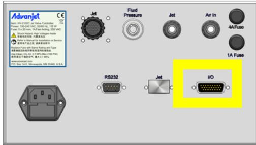
The I/O connector is a 26-pin, high-density, D-SUB, board-mounted receptacle (female sockets). This HD26 I/O connector connects to one type of input circuit and four types of output circuits. The design notes suggest at least one interface circuit on the user's side of each type of input or output.
