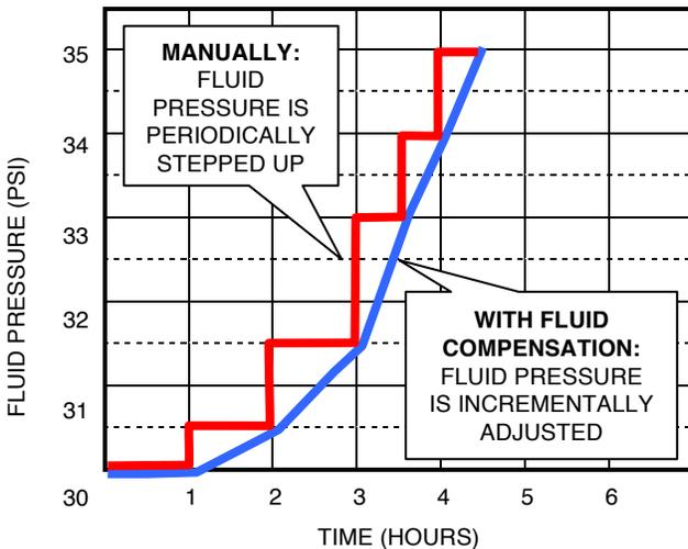
Figure 4-12: Fluid Pressure Adjusted Over Time
