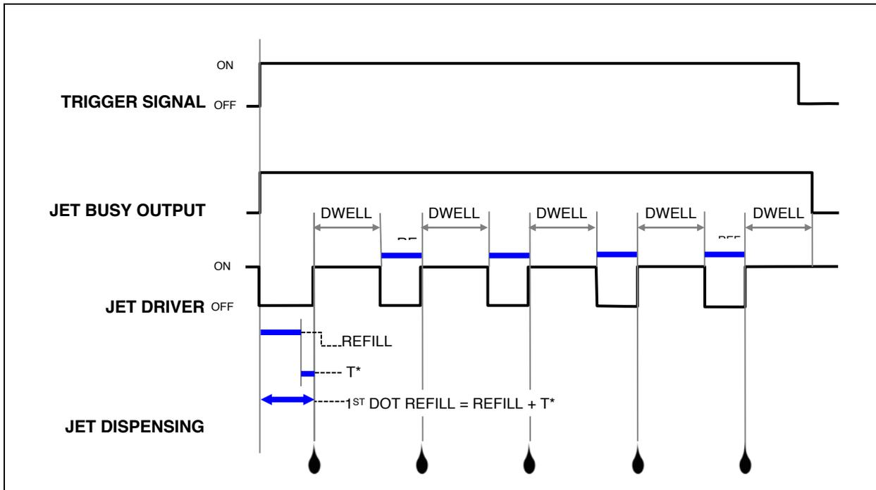
Figure A3- 2: 1<sup>st</sup> Drop Compensation in LEVEL Mode, # of Drops = 1
