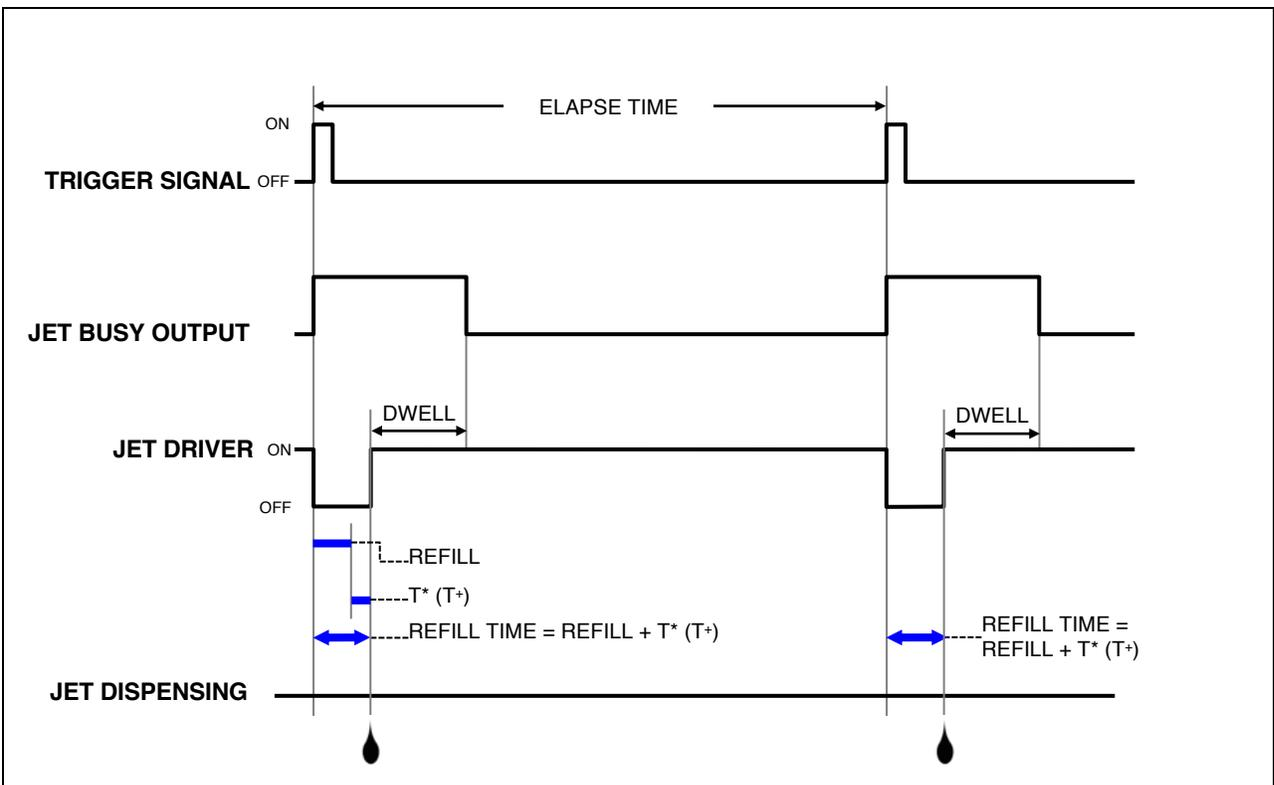
Figure A3- 1: 1<sup>st</sup> Drop Compensation in PULSE Mode, # of Drops = 1
