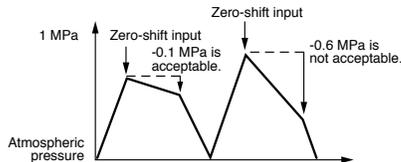
When the power is turned off, the value updated after the zero-shift input (zero-shift value) is lost.
