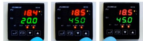
Figure 3-8: Press
