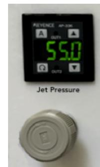
Figure 3-4: Jet Pressure Gauge and Regulator
