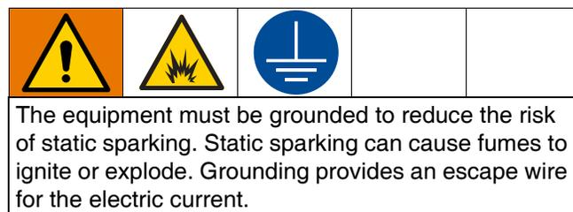
**Pump:** use the ground wire and clamp provided. Verify that the ground screw is attached and tightened securely to the bottom of the air motor. Connect the ground clamp to a true earth ground
