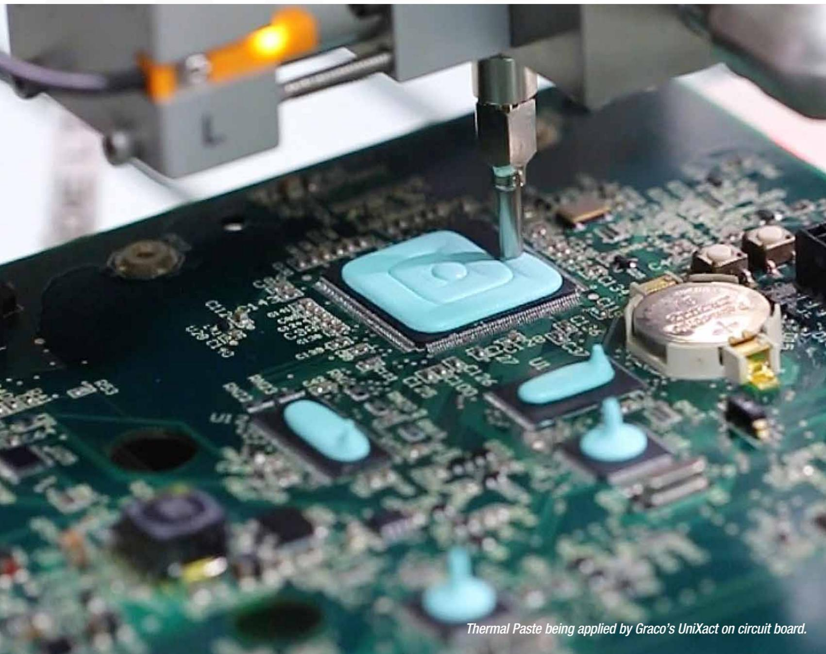
*Thermal Paste being applied by Graco's UniXact on circuit board.*
